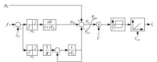
Figure 16: : La Gomera flywheel active power-frequency controller.
