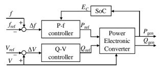
Figure 12: La Palma ultra-capacitor high-level model.
